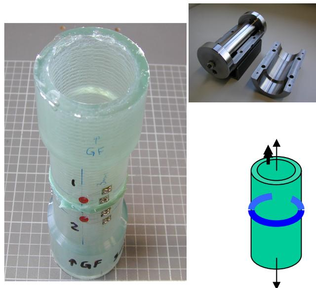
**Figure 8: Tubular specimen for bonding paste shear testing, mould and loading concept**
