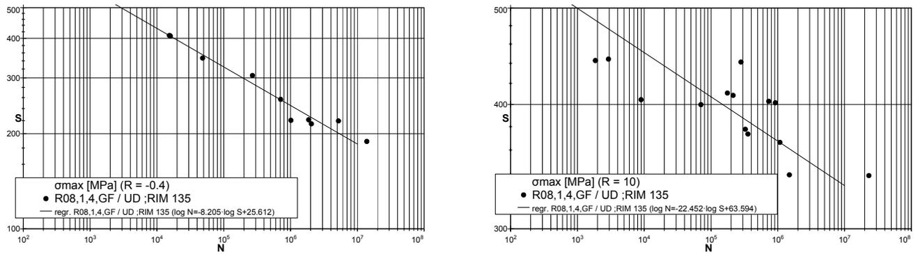
Figure 4: S-N data used to construct Figure 3
