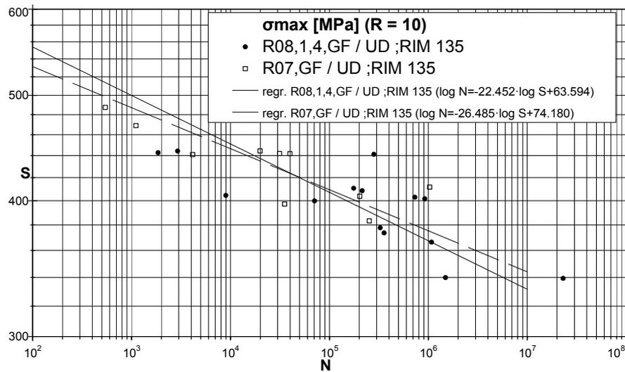
Figure 5: Comparison of 2 different specimen geometries at R = 10
