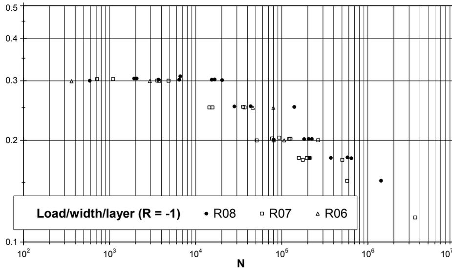
**Figure 1: Comparison of fatigue behaviour for three different geometries. (For R08 see Figure 3; R06 is 25 mm wide, R07 has gauge length of 30 mm and is 6 layers)**
