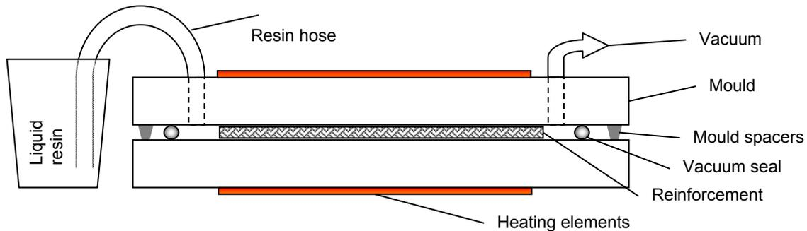
**Figure 2: Mould for reference specimen production**
