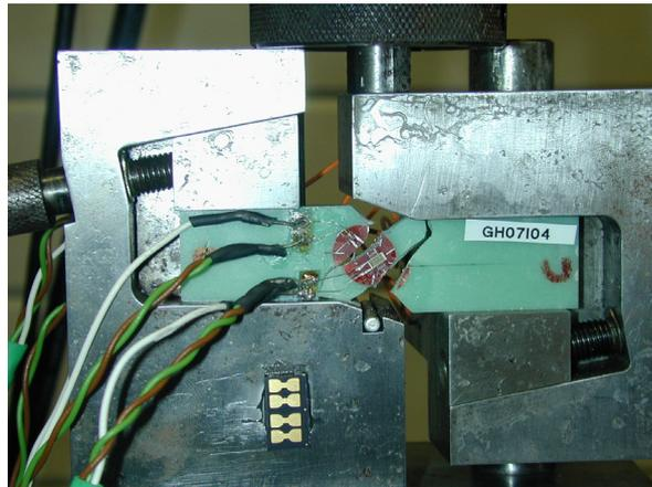
**Figure 9: Shear strength testing on bonding paste**
