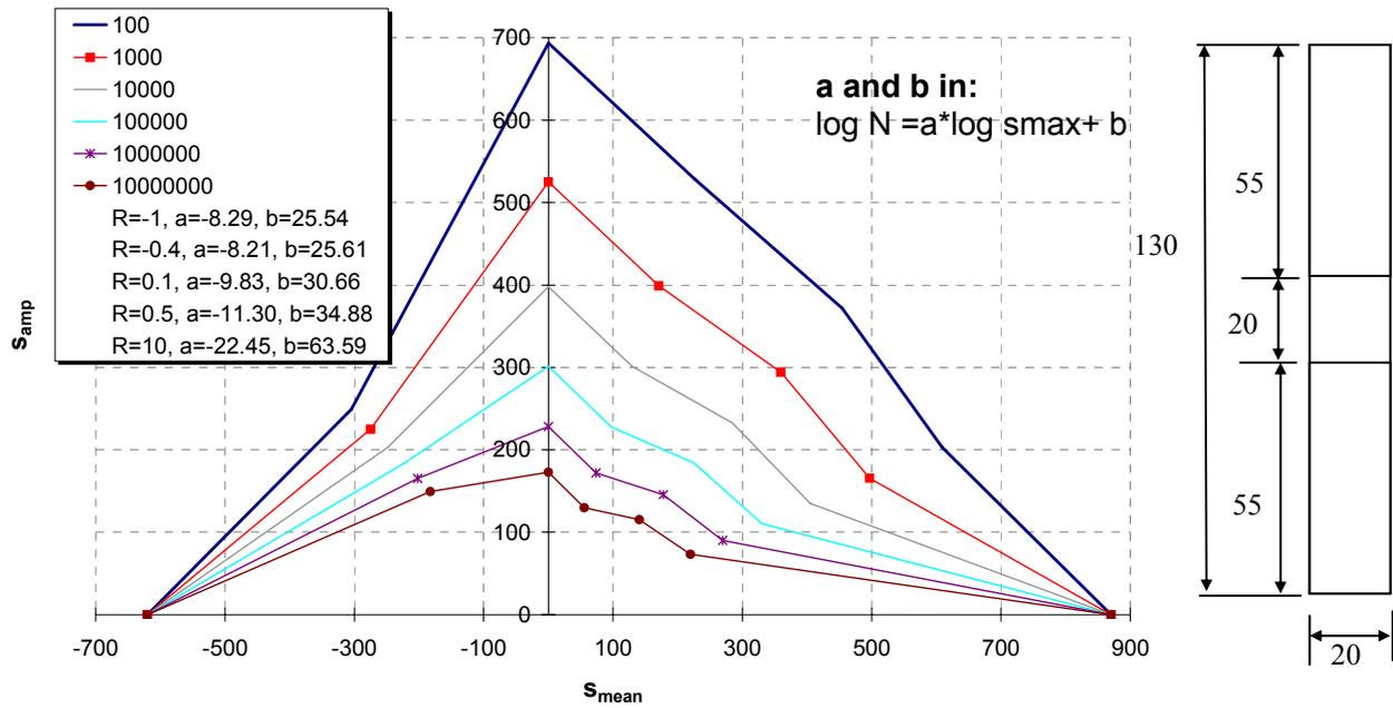
**Figure 3: Constant life diagram of reference material, R08 geometry**
