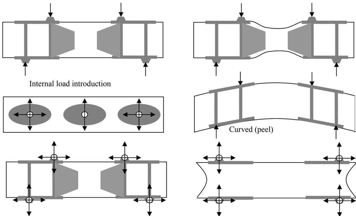
**Figure 7: Candidate I-beam concepts (side view; arrows indicated loading direction, grey areas indicate extra reinforcement)**
