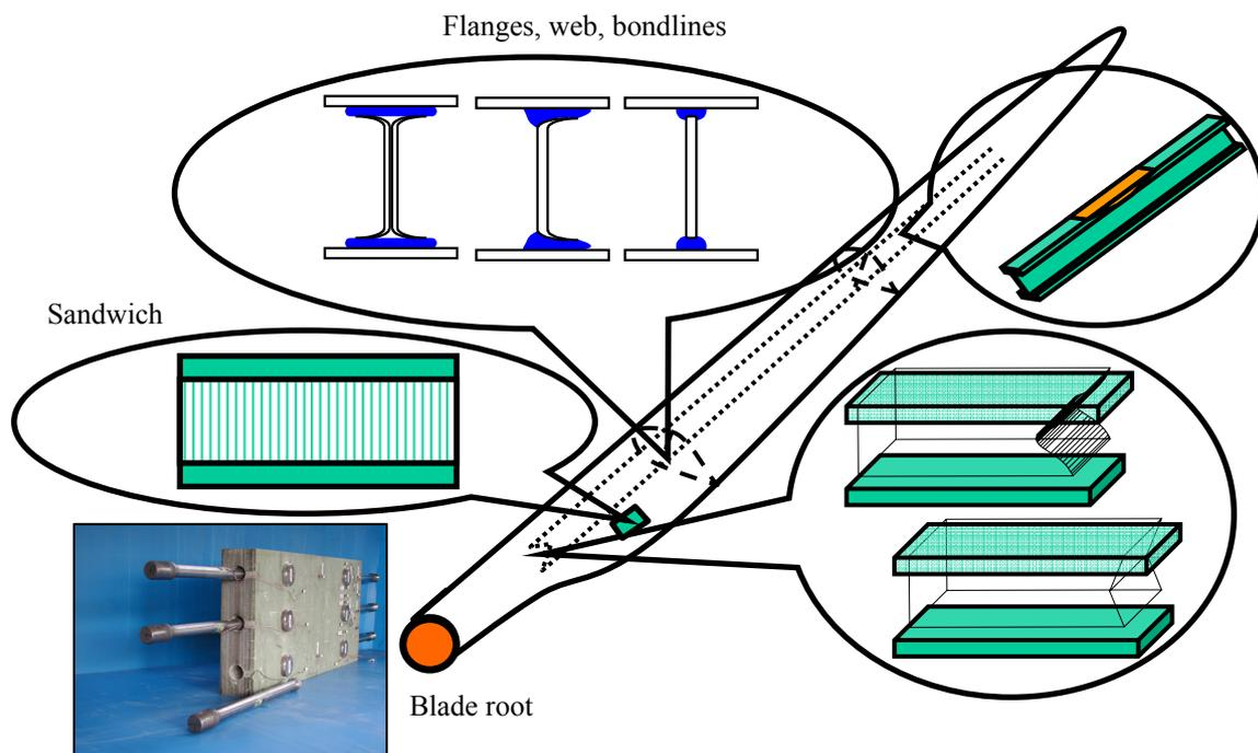
**Figure 6: Parts of blade represented in subcomponents**
