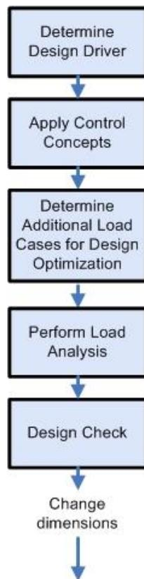
Figure 7.2: Adapted support structure design process
