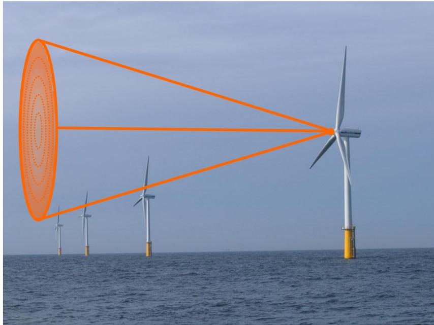
Figure 5.11: Principle of a nacelle-mounted LIDAR (background Figure *Econcern*)
