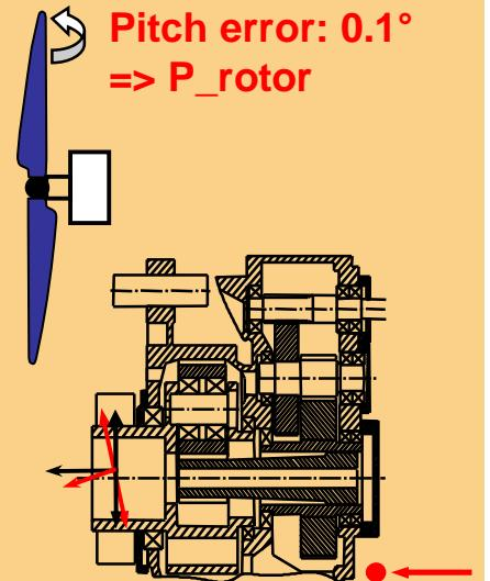
Main shaft & planet carrier coupling misalignment:
