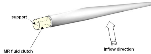
Figure 13: Wind tunnel experiment with the torsional clutch
